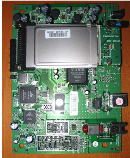
Figure 8.19: Helium chip as part of a home gateway ADSL modem (partially masked by 802.11 module).
