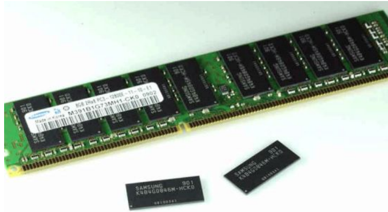
Figure 13.8: DRAM single-in-line memory module (SIMM).
