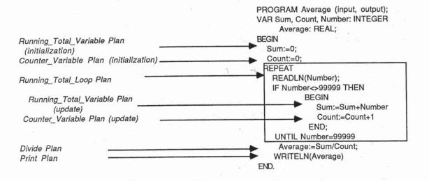
Figure 1: Representations of a program computing an average.
