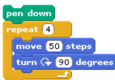
Fig. 3. Lesson-4, showing a repeat-block for iteration
