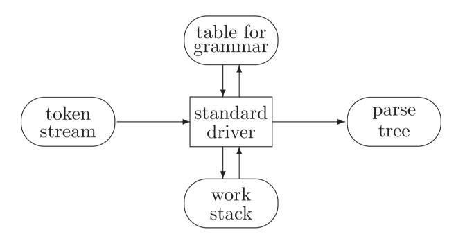
In LR parsing, the table represents the *characteristic finite state* machine (CFSM) for the grammar; the standard driver (grammar independent) merely interprets this.
