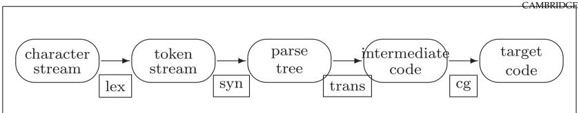
A classical compiler does all these on one machine. To distribute a system for multiple architectures we compile it once per architecture.
