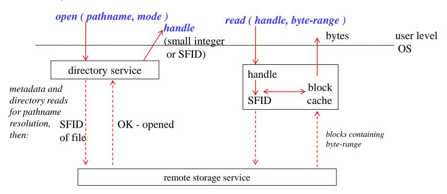
If the SS is stateless it does not support **open** at its interface and holds no info on files in use.
