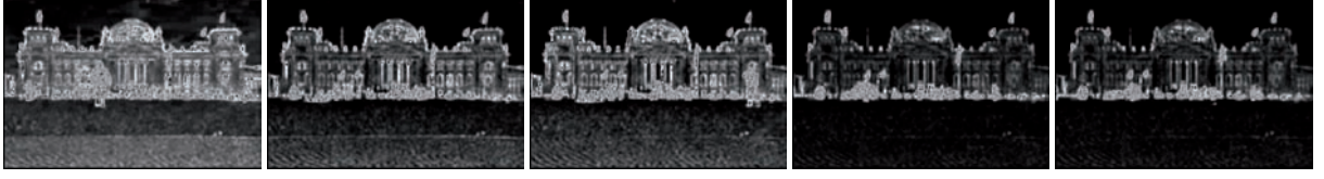
Figure 4: The confidence images for the set of input images for the Reichstag set of images, computed based on 7 \times 7 neighborhood patches. Darker pixels reflect small distance to the model represented by the image set and, thus, high confidence. Conversely, light pixels depict low confidence. Only the first five out of seven source images are shown.
