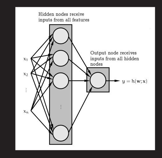
For the output:  $\sigma(a) = a$ . For the hidden nodes  $\sigma(a) = \frac{1}{1 + \exp(-a)}$ .
