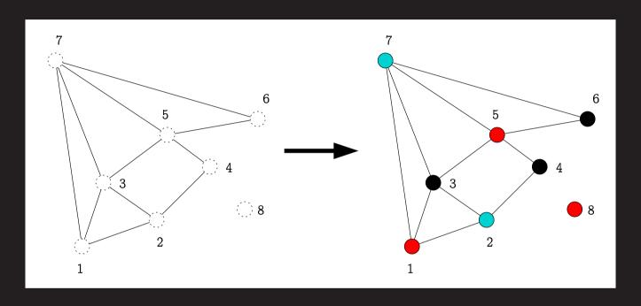
Each node corresponds to a *variable*. We have three colours and directly connected nodes should have different colours.
