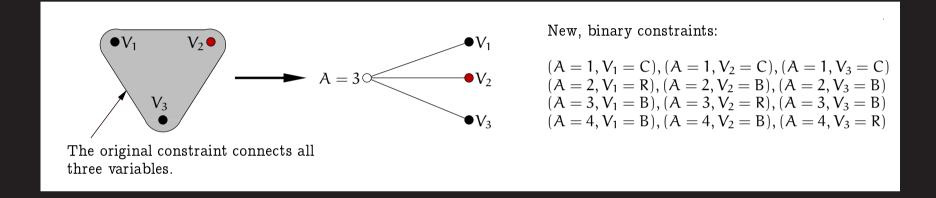
Introducing auxiliary variable A with domain  $\{1, 2, 3, 4\}$  allows us to convert this to a set of binary constraints.
