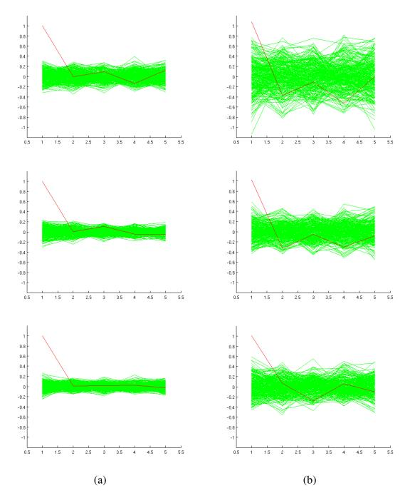
Fig. 10. Results of CPA (a) and DPA (b), for m=100 (top), m=1000 (middle) and m=100000 (bottom). The X-axis represents the 5 iterations of each encryption operation in our algorithm; the Y-axis represents the amplitude of the correlation for CPA and the amplitude of the differential trace for DPA
