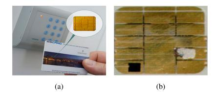
Fig. 1. Smartcards: (a) a smartcard used in access control; (b) a tampered smartcard
