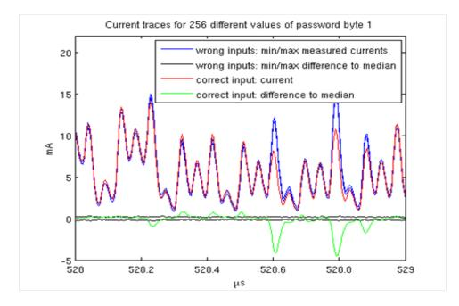
Fig. 4. SPA attack on the MC68HC908AZ60A microcontroller: plotting the intensity for all 256 possible values of a password-byte it is possible to determine the out-lier which corresponds to the correct byte; figure from [3]
