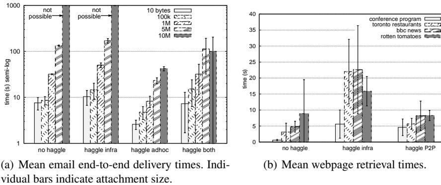
Fig. 4: Email and web experiment performance. Both graphs show standard deviations as error bars. Lower values are better. Note that in 4(a) for both *no hagggle* and *hagggle infra* cases it was not possible to send 10M emails due to server limitations. 4(b) does not show *no hagggle P2P* because it is not possible to access web pages using existing software.
