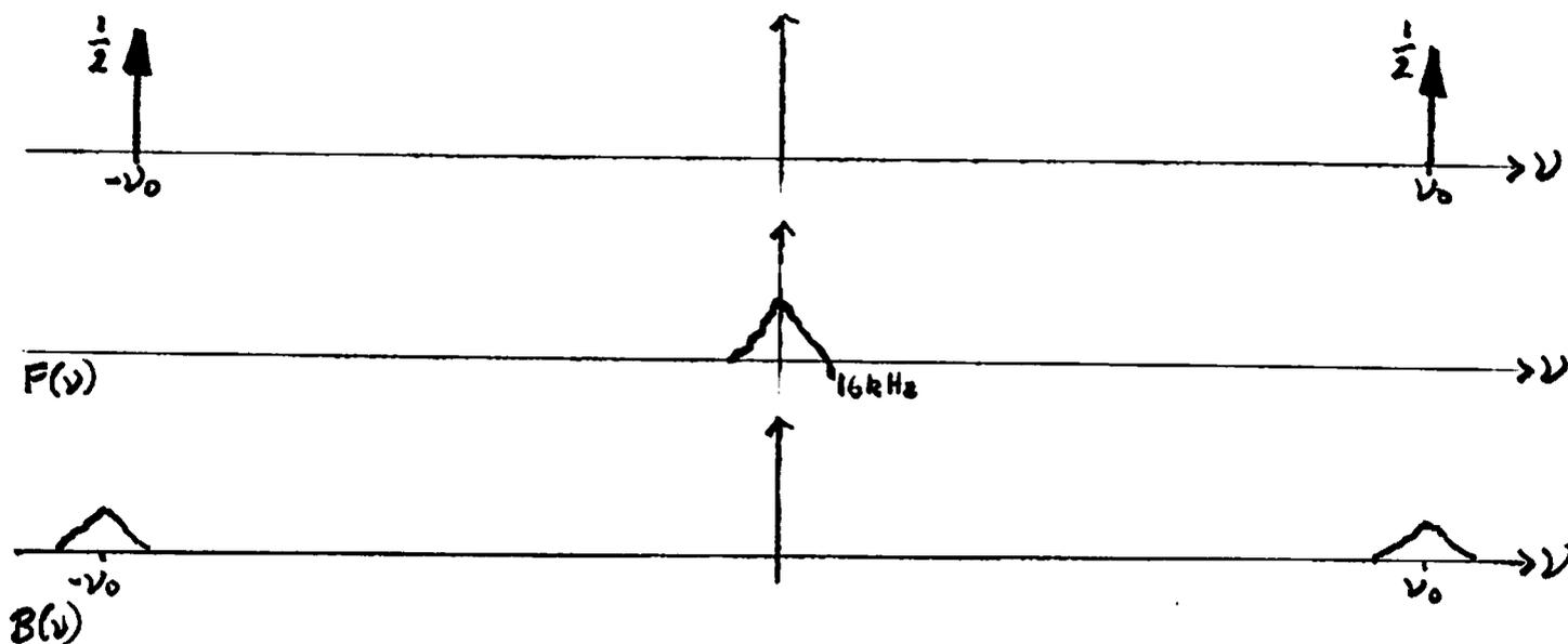
How do I now recover the original signal? It's simple: I simply multiply  $b(t)$  by a sinusoid of the same frequency:
