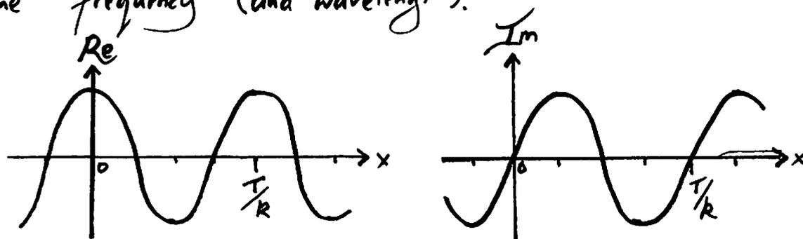
If we now plot this on the Argand diagram (three axes:  $x$ ,  $Re$ , and  $Im$ ) we get a curve which stays a constant distance from the  $x$ -axis and spirals around the axis like a corkscrew.
