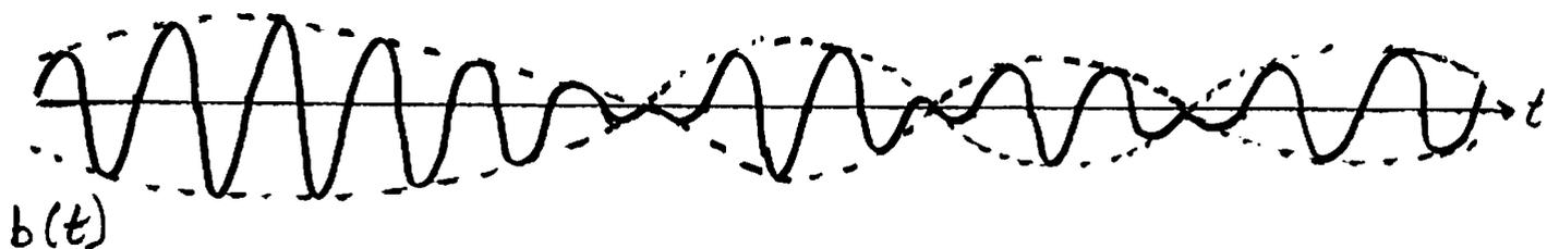
What happens in the frequency domain? Well, the F.T. of  $f(t)$  is CONVOLVED with the F.T. of the sinusoid.
