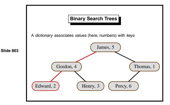
Binary search trees are an important application of binary trees. They work for keys that have a total ordering, such as strings. Each branch of the tree carries a (key, value) pair; its left subtree holds smaller keys; the right subtree holds greater keys. If the tree remains reasonably balanced, then update and lookup both take  $O(\log n)$  for a tree of size n. These times hold in the average case; given random data, the tree is likely to remain balanced.
