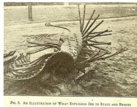
FIG. 5. AN ILLUSTRATION OF WHAT EXPLOSION DID TO STAYS AND BRACES
