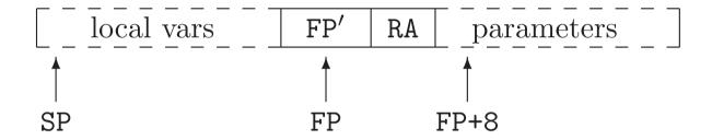
Space below (to the left of) the stack frame is used to construct the argument list (possibly empty) of any called routines—the called routine then turns this into a 'proper' stack frame.
