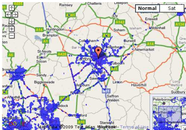
Figure 12: Skyhook’s coverage of Cambridge. Each blue dot is a logged WiFi point and position.
