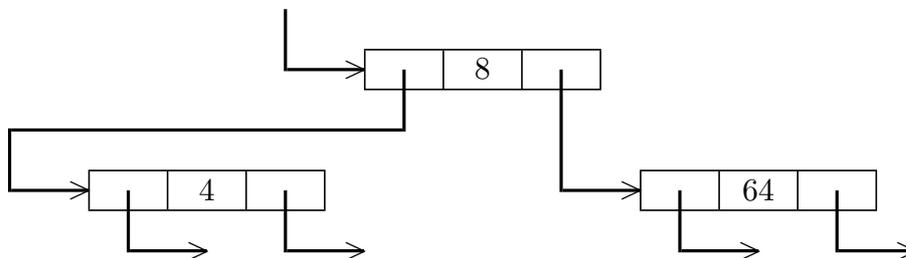
The tree is built up one node at a time. A new node is put on the tree in such a way that the tree is ordered. Thus  $4 < 8 < 64$ . If the next new node is to incorporate 32, it will hang from the left of the 64 node.
