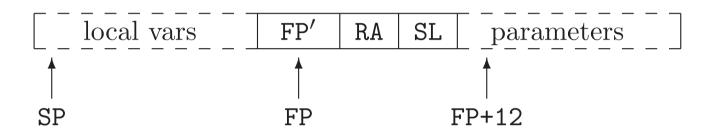
SL is the 'static link'—a pointer to the frame of the *definer* Note that FP' is a pointer to the frame of the *caller*.
