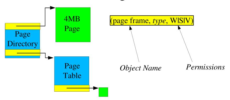
Note that the *type* field was always latent, implied by containership in a structure (the page table/page directory) that contained typed slots
