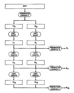
The key schedule of DES breaks the key into two 28-bit halves, which are left shifted by two bits in most rounds (only one bit in round 1,2,9,16) before 48-bit are selected as the subkey for each round
