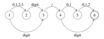
Accept states are shown with a double circle. This is a non-deterministic FSA: for instance, an input starting with the digit 3 will move the FSA to both state 2 and state 3. This corresponds to a *local ambiguity*: i.e., one that will be resolved by subsequent context. By convention, there must be no 'left over' characters when the system is in the final state.
