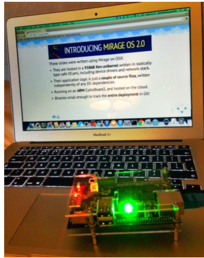
A Mirage web server unikernel running as a Xen guest on an ARM CubieTruck serves up a slide deck.
