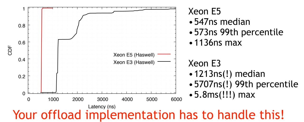
Netronome NFP-6000, Intel Xeon E5-2637v3 @ 3.5GHz (Haswell) Netronome NFP-6000, Intel Xeon E3-1226v3 @ 3.3GHz (Haswell)
