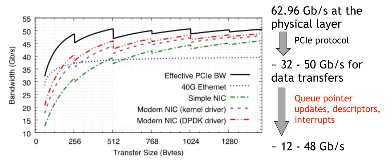
Model: PCIe gen 3 x8 64 bit addressing
