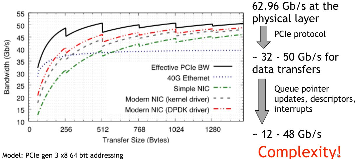
Model: PCIe gen 3 x8 64 bit addressing
