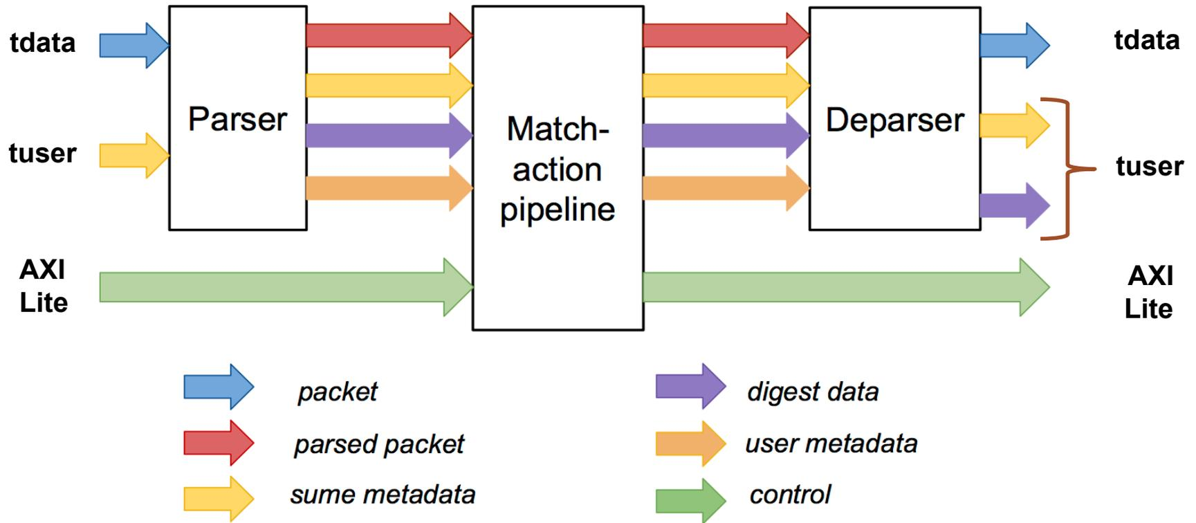
P4 used to describe parser, match-action pipeline, and deparser
