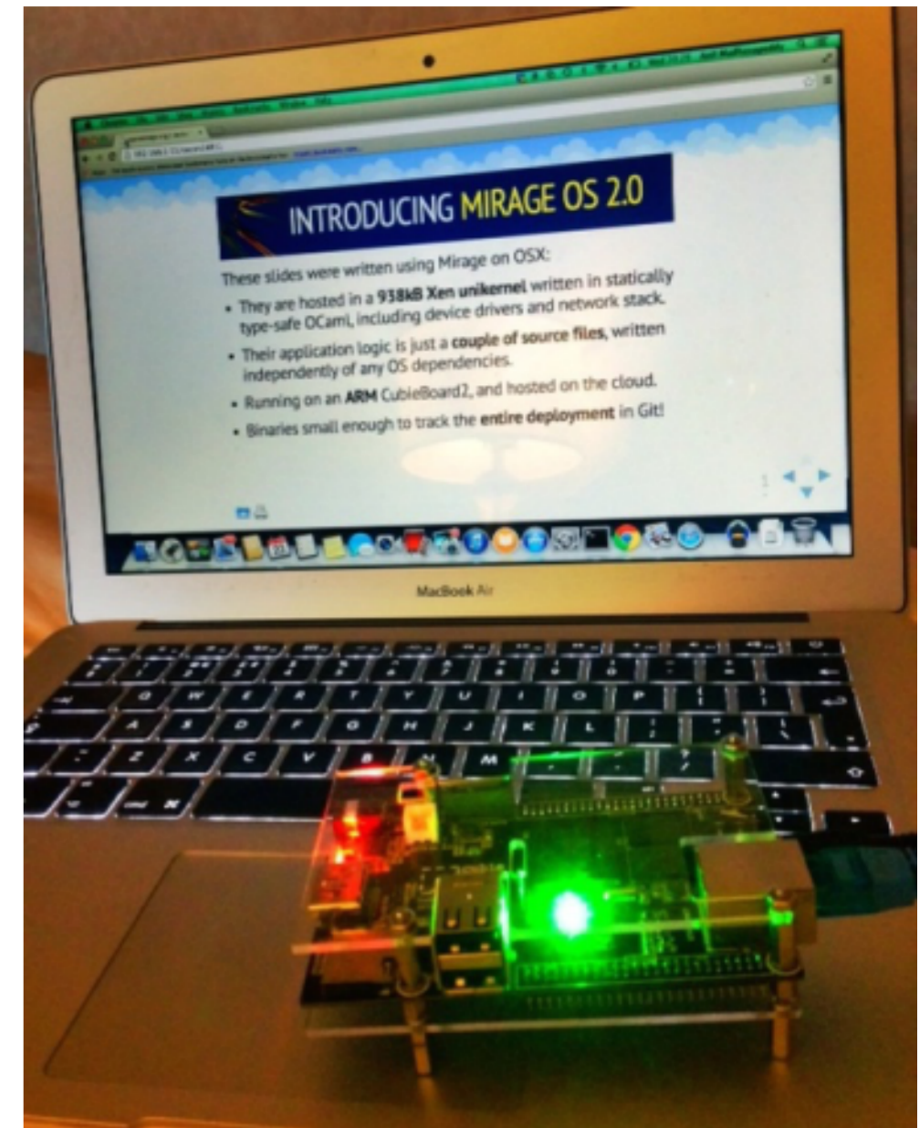
A Mirage web server unikernel running as a Xen guest on an ARM CubieTruck serves up a slide deck.
