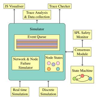
Figure 1: Overall architecture of our simulator.
