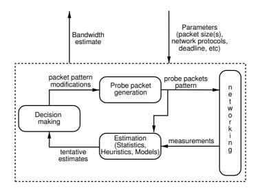
Fig. 1. Design scheme of an active bandwidth estimation tool
