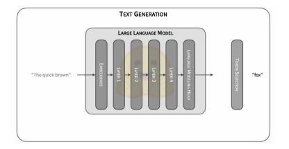
The autoregressive generation of decoder-only Transformer models can be decomposed in two phases.
