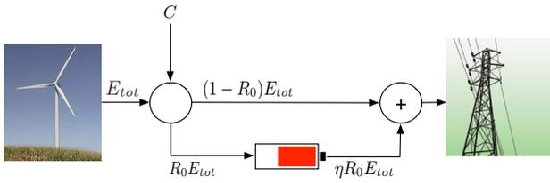
Figure 9: **Simple model used in [6]:** Idealized storage assumption ( $B = \infty$ ,  $\alpha_c, \alpha_d = \infty$ , and  $\gamma = 0$ ) and no access capacity constraint on the power transmitted from the storage.
