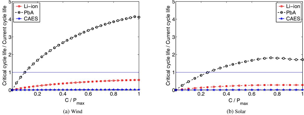
Figure 8: The ratio of critical cycle life to current cycle life for different storage technologies with  $B = 10\text{MWh}$ : The cycle life must be scaled by these values for the storage devices so that they are sufficiently energy efficient to replace curtailment.
