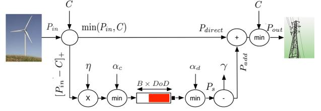
Figure 3: **Integrating renewables using storage devices:** Using a non-ideal storage device with parameters  $(\alpha_c, \alpha_d, \eta, DoD, B, \gamma, \lambda)$  to transfer renewable power  $P_{in}$  over an access line, with maximum allowable power transmission of  $C$ .
