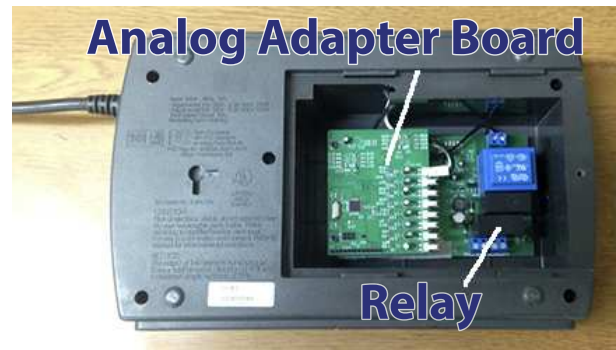
Figure 5: The internals of an Emonix smart power strip include a relay to switch power to the plugs it serves and an analog adapter board to sense the power consumption of the connected appliances. The main CPU sits beneath the analog adapter board along with its WiFi interface that directly connects to the home’s network. This allows energy measurements to be relayed to an off-site controller.
