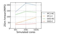
Figure 7: Performance distribution of single-thread zsim on SPEC CPU2006, using four models: IPC1 or OOO cores, with and without contention (C/NC).
