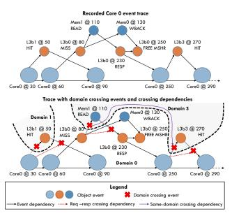
Figure 4: Example event trace from bound phase (of core 0 in Figure 3), and its division in domains with domain crossing events inserted for simulation in the weave phase.
