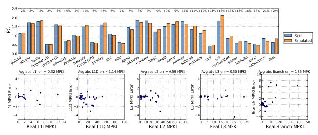
Figure 5: Validation of the OOO core model against a real Westmere machine on SPEC CPU2006: Simulated vs real IPC, and scatter plots of per-application MPKI errors (simulated - real MPKI) for all the caches and the branch predictor.
