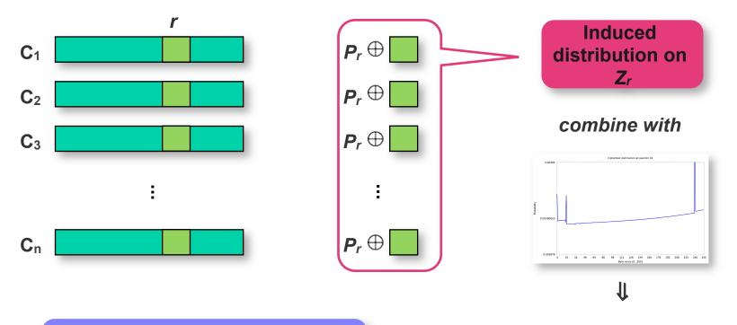
Recovery algorithm: Compute most likely plaintext byte Likelihood of *P<sub>r</sub>* being correct plaintext byte
