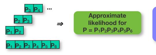
**Recovery algorithm:** Viterbi-style algorithm to determine P with highest approximate likelihood
