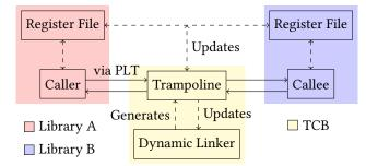
The diagram above illustrates the interaction between various elements during a inter-library function call when compartmentalisation is enabled. The trampoline intercepts the control flow both during call and return, but is intended to be completely transparent to the software. It pushes the return address to the trusted stack and updates the content of the register file, including switching the stack pointer.
