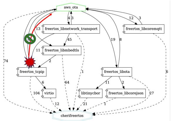
CheriFreeRTOS components and the application execute in compartments. CHERI contains an attack within TCP/IP compartment, which access neither flash nor the internals of the software update (OTA) compartment.
