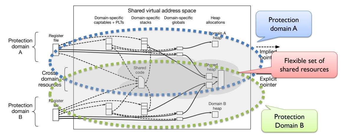
Isolated compartments can be created using closed graphs of capabilities, combined with a constrained non-monotonic domain-transition mechanism
