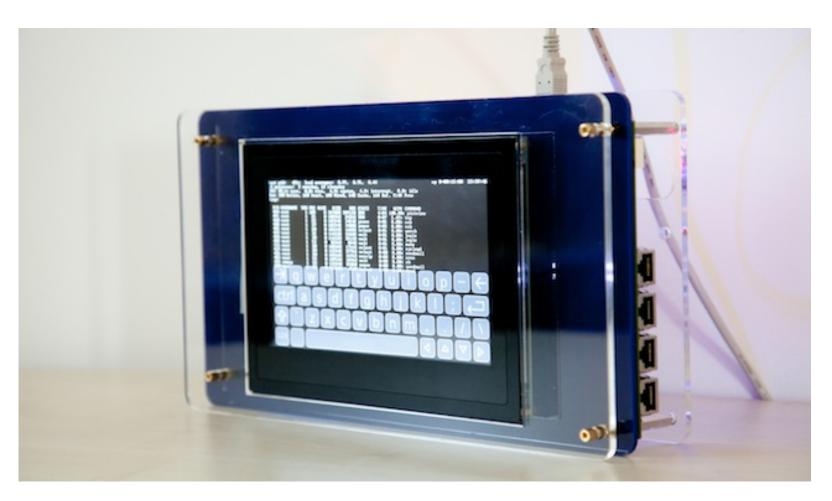
Terasic DE-4 tablet hosting 100MHz CHERI processor, CheriBSD OS
