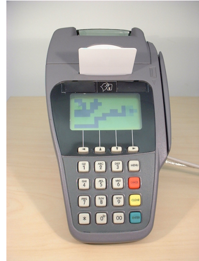
(b) Customer's view of terminal. Here, it is playing Tetris, to demonstrate that we have full control of the display and keypad.
