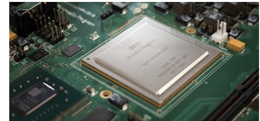
High-performance Arm Morello chip able to run a full CHERI software stack, Cambridge, 2022
