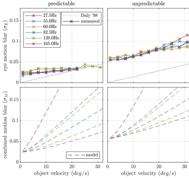
Fig. 15. Top: blur  $\sigma$  based on eye tracker data for a range of refresh rates (different colors) and object velocities (x-axis). Blur was computed over 25ms intervals as the distance traveled by the tracked object on the retina. Dotted line: Daly's model. Bottom row: model predictions for blur taking into account both eye motion and display hold-type behavior.
