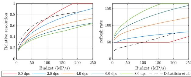
Fig. 21. Model predictions for predictable motion for different velocities (colors) in  $\text{deg/s}$  (dps) plotted against Debattista et al. [2018] (dashed line). Assuming viewing distance of 108 cm and a field of view of  $30^\circ$ . Resolution is relative to linear image size; Refresh rate predictions are for QHD resolution.
