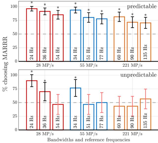
Fig. 23. Results of validation experiment showing the percentage of participants picking the proposed adaptive MARRR algorithm over standard *constant-resolution-and-constant-refresh-rate* rendering, viewing predictable (top) and unpredictable (bottom) motion. Colors denote different rendering budgets. The refresh rates were selected around the predictions of [Debatista et al. 2018]. Error-bars denote 95% confidence intervals.
