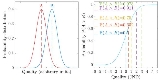
Fig. 4. Left: the quality of two conditions A and B is represented as two normally distributed random variables. Right: a pairwise comparison experiment let us measure  $P(A > B)$  or  $P((A - B) > 0)$ . We use a cumulative normal distribution to recover the quality difference from such probability. The plot shows how JND values correspond to the portion of a population selecting condition A over B. Negative scores indicate that the quality of A is worse than the quality of B.
