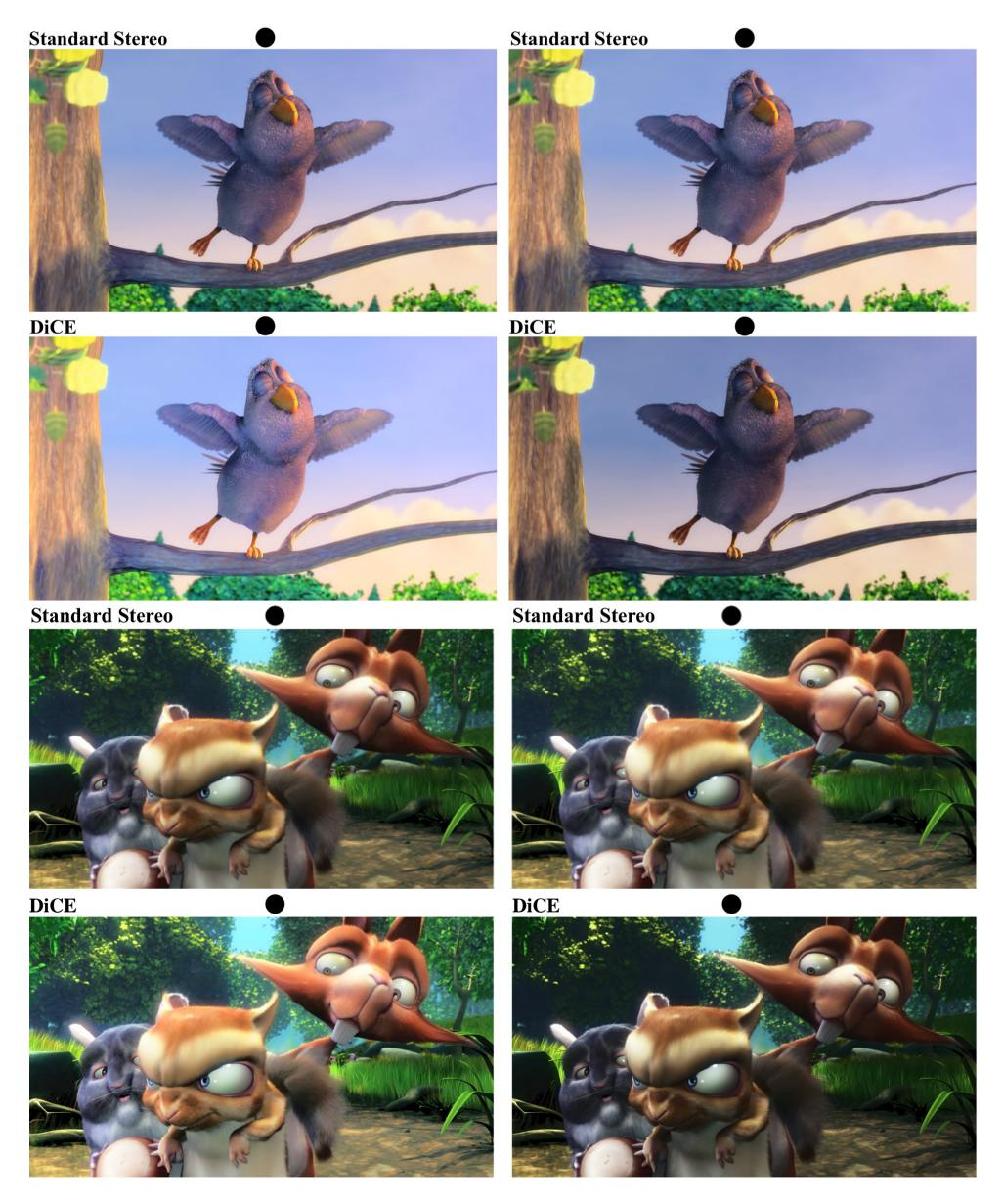
Comparison of standard stereo images and the images with enhanced perceived contrast using our DiCE method. They can be cross-fused with the assistance of the dots above the images. Notice the enhanced contrast in the shadows and highlights of the scene.
