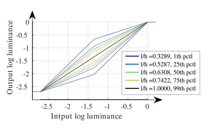
The shape of the dichoptic tone-curves at different l/h ratios. The ratios were selected to represent 1st, 25th, 50th, 75th and 99th percentile of the data (across all images and observers) from our experiment.
