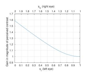
Fig. 7. The gain in contrast due to fusing left and right eye images which are processed by the tone curves with the slopes  $s_l$  and  $s_h$  (x-axis). As the tone curve slope is reduced on the left eye ( $s_l$ ), it is increased on the right eye ( $s_h$ ). Such a change in slope does not reduce the dynamic range budget allocated to both eyes, but it boosts fused contrast.
