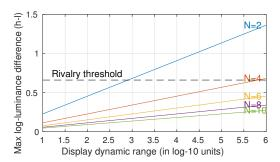
Fig. 14. The maximum log-10-luminance difference (h - l) for a given display dynamic range (x-axis) and the number of segments (N, colors). The plots are drawn assuming l/h = 0.63 (50th percentile). The dashed line represents the rivalry threshold (50th percentile) for log-luminance difference (Experiment 1b, in supplementary). The plot shows that for most SDR displays (dynamic range <2.8 log-10 units), we do not need more than 2 segments.
