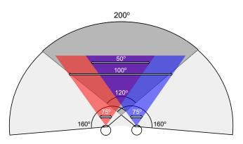
Fig. 3. Arcs denote angles for viewing in the real world: each eye sees a field of view of about 160°. This results to a 200° combined horizontal field of view, 120° of which are overlapping and thus binocular processing or stereopsis is possible. Two-headed arrows denote angles in a modern VR headset: each eye sees a horizontal FoV of about 75°, leading to a 100° combined FoV, only 50° of which are overlapping and available for binocular processing or stereopsis.
