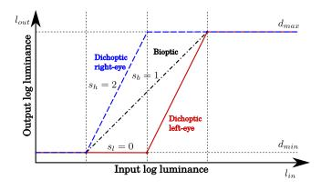
Fig. 6. When a separate tone curve is used for each eye (dichoptic presentation) the slope of one of the curves can be up to twice as high as that for a standard dioptic presentation. The perceived contrast for the dichopic images will be 10%-50% higher (see Figure 7). However, such strong separation of the tone curves will result in an image that is very uncomfortable to view.
