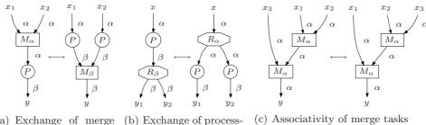
(a) Exchange of merge (b) Exchange of process- (c) Associativity of merge task and processing tasks ing and replication tasks
