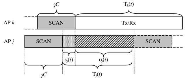
Fig. 4. Fraction of  $T_j(t)$  overlaps  $T_k(t)$  and SCAN portion of AP  $k$ .
