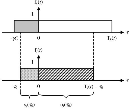
Fig. 5. Representation of MAC frames as unit step functions.
