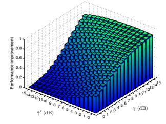
(Left-hand side) Effect of the network parameters on the performance gain for a target PEP of  $10^{-2}$ . (Right-hand side) Theoretical performance improvement that optimal power allocation can achieve over equal power allocation for a network of  $M=4$  users.
