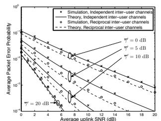
Comparison between analytical values and simulation results when the rate  $\frac{1}{2}$  NRNSC(15, 17) code is used. The network size is  $M=2$  (left-hand side) and  $M=4$  (right-hand side).
