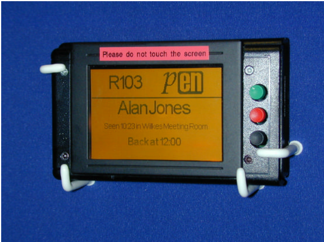
Figure 6. PEN display node acting as a door sign.
