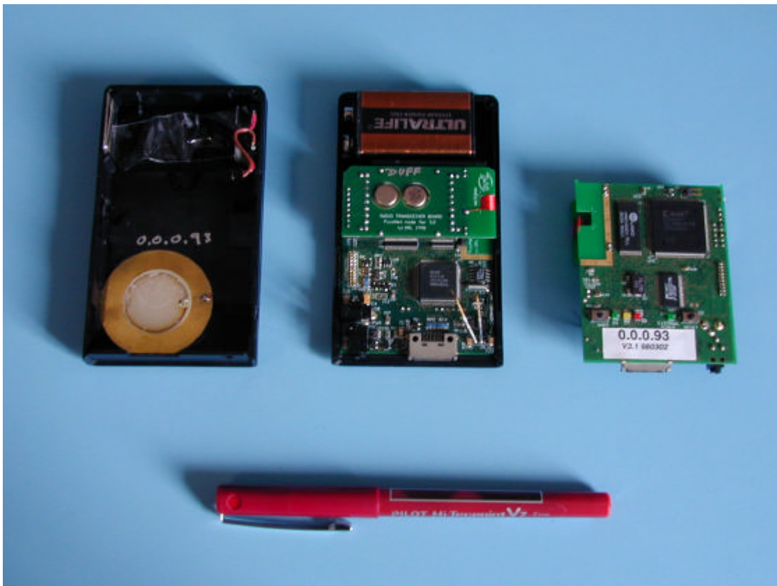
Figure 1. Both sides of a PEN node, and a pen.
