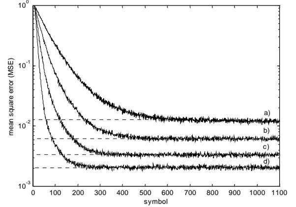
Fig. 2: convergence rate for SUI-2, ULA( $0.5 \lambda$  spacing), DOA spread  $3^\circ$ : a) 1 antenna, b) 2 antennas, c) 4 antennas and d) 8 antennas
