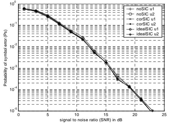
Fig. 6: probability of symbol error (Ps) for equal power users (i.e. SIR=0dB)
