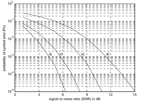
Fig. 3:  $P_s$  for one user system: a) 1 antenna, b) 2 antennas, c) 4 antennas and d) 8 antennas
