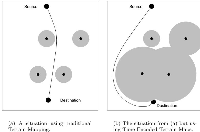
Figure 1: An example situation where navigation using traditional Terrain Mapping may produce erroneous paths by not accounting for obstacle dynamics while using Time Encoded Terrain Maps anticipates obstacle dynamism and routes around potential impediments.
