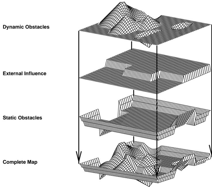
Figure 2: The Terrain Map is formed by the successive superposition of several layers in increasing order of rate of change.
