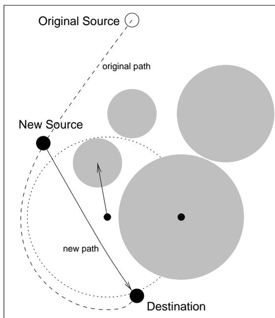
Figure 5: Recalculation of the path during execution allows for refinement to account for actual known motion of the obstacles
