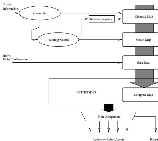
Figure 7: Cooperation Planner structure illustrating the core use of Time Encoded Terrain Maps to fuse multiple data sources and extract a unified strategy.
