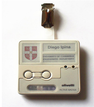
Fig 2 Containment: Active Badge
