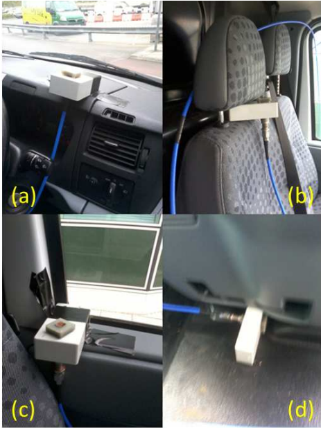
Fig. 5. NPL Van: (a) Unit 1 - dashboard; (b) Unit 2 - middle seat headrest; (c) Unit 4 - passenger door; (d) Unit 3 - middle floor.
