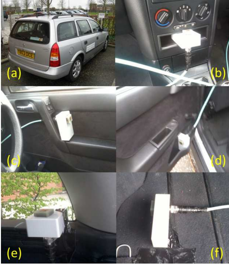
Fig. 4. Lab Car: (a) Car; (b) Unit 1 - dashboard; (c) Unit 2 - front driver side door; (d) Unit3 - rear passenger side door; (e) Unit 4 - boot driver side window;- (f) Unit 5 - boot passenger side floor.
