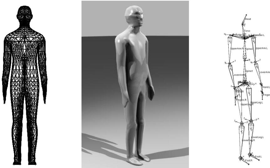
Figure 2.5: Alfred, one of the meshes used as input data. From left to right: The triangle mesh in wire-frame view; a raytraced perspective view; and the skeleton in its rest position.
