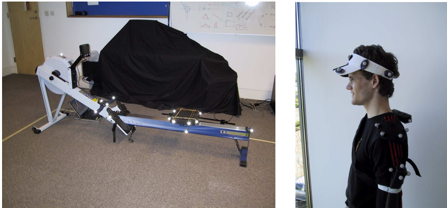
Fig. 1. Ergometer and rower augmented with VICON markers. The erg, its seat and its handle were 3 objects. Parts of the body were captured for future use.
