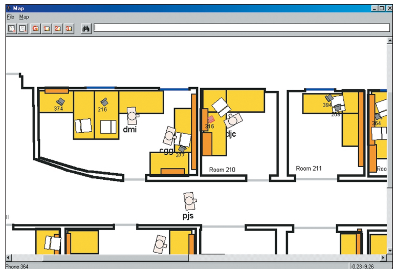
Figure 4. A 2D-map visualization of the world model. In Room 210, a user (djc) is sitting in front of his workstation while using his telephone, which is colored red to indicate that it is off the hook.
